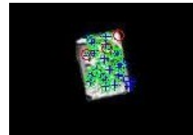
Fig. 2. Each point in the figure corresponds to the location of an extracted SIFT feature. This is a training example of a cereal box used for recognition. Note the numerous number of feature points due to the complex texture on the cereal box.
