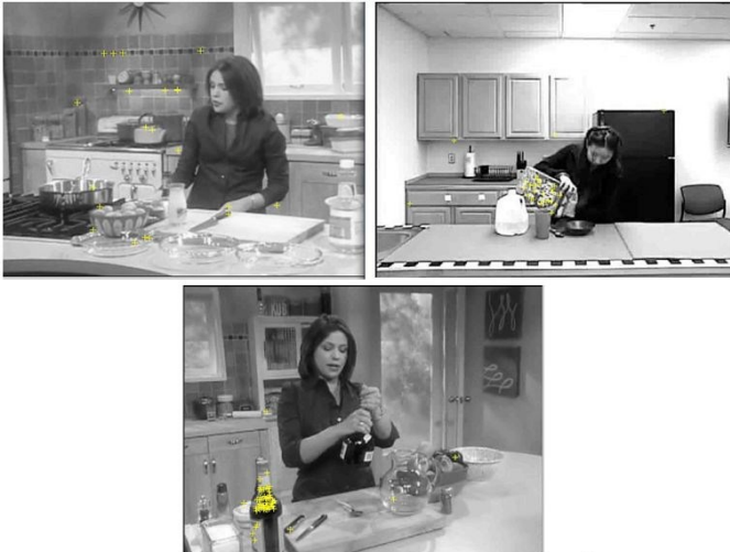
Fig. 11. SIFT features, represented by yellow + signs, found to match the model of the knife (top left), the cereal box (top right), and the wine bottle (bottom). Note the large number of matched SIFT features for the cereal box because of its large amounts of texture, and the small number for the less textured knife.
